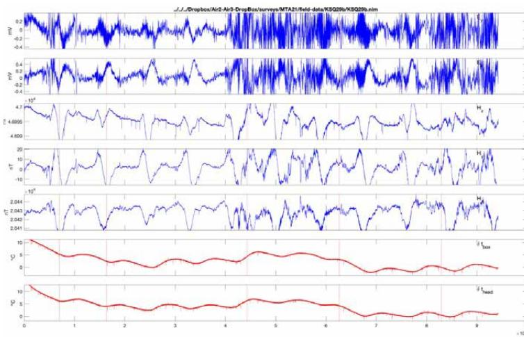
(LEFT) Time-series containing 11-d of ground-level electric field (from top-to-bottom: N-S component of E field, E-W component of E field, N-S component of B field, E-W component of B field, vertical component of B field; red curves are sensor and DAQ system temperatures).
