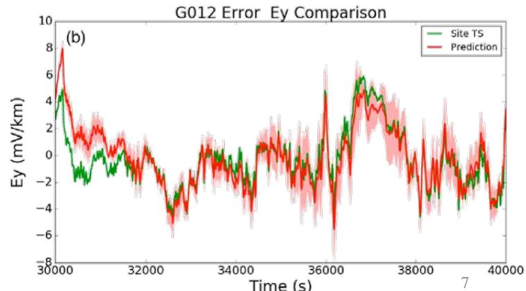
Given measurements, predictions or forecasts of ground-level electric fields, the vector E fields can be integrated along the power transmission grid line paths and the space weather induced bus voltages used as inputs to an AC/DC powerflow solution – PowerModelsGMD.jl to determine GICs
