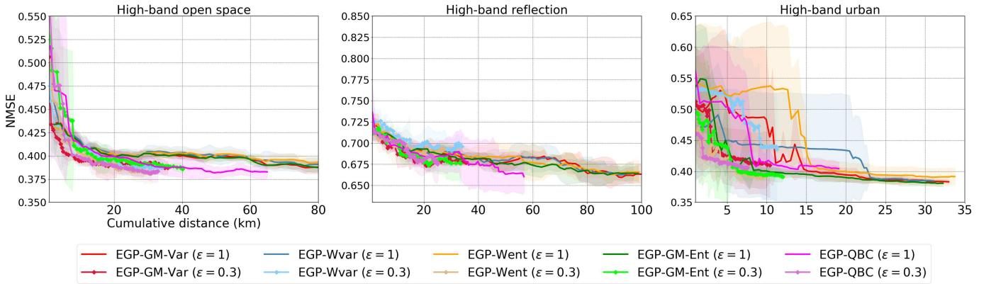
Fig. 8: NMSE vs cumulative distance 26GHz high-band data under (a) high-band open space; (b) high-band urban canyon; and (c) high-band reflect datasets.
