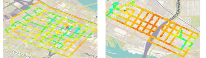
Fig. 3: Radio coverage maps for real RSS measurements. Green color represents strong RSS, while red poor RSS.
