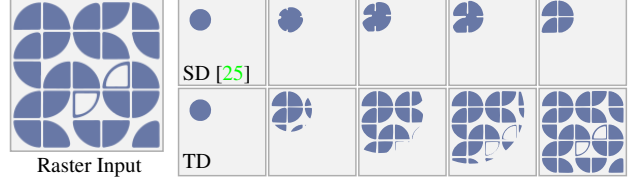
Figure 3. Reconstruction of vector images from raster input. Shape derivatives (analogous to curve gradients in [25]) evolve closed curves with visibility changes only on the boundaries. These gradients are sparse and the optimization can plateau at a local minimum (top). Topological derivatives can reconstruct a vector image (bottom) from a raster input (left) with adaptive topological changes.
