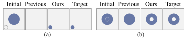
Figure 1. Pathologies of shape derivatives. Previous work on inverse surface reconstruction relies on shape derivatives which are inadequate for instances when (a) the target geometry is far from the initialization, and when (b) target has a hole in the interior. We resolve these failure cases with topological derivatives.
