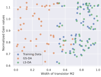
Figure 5. Simplified illustration of the coverage of the normalized sizing solution space (consisting of only the width of transistor M2 in Figure 3(a)) for the two-stage differential amplifier. GS-DA achieves global long range coverage far away from the training sizing solution data, while LS-DA achieves local coverage around the training data.
