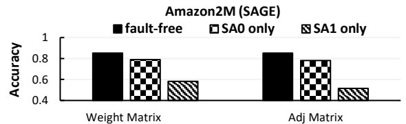
Fig.3. The accuracy of trained model after introducing 5% SA0 or SA1 pre-deployment faults on the weight and adjacency matrix separately.
