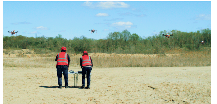
Fig. 2. Using the DroneResponse platform, multiple sUAS fly autonomously in close vicinity to one another, requiring safe minimum separation distances to be maintained at all times.
