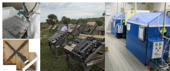
Figure 1: Standard Corrosion Science Experiment: Each material is manufactured into sample panels (Left Top). They are assessed (Left Bottom) after being exposed to indoor (Right) or outdoor (Middle) environments.
