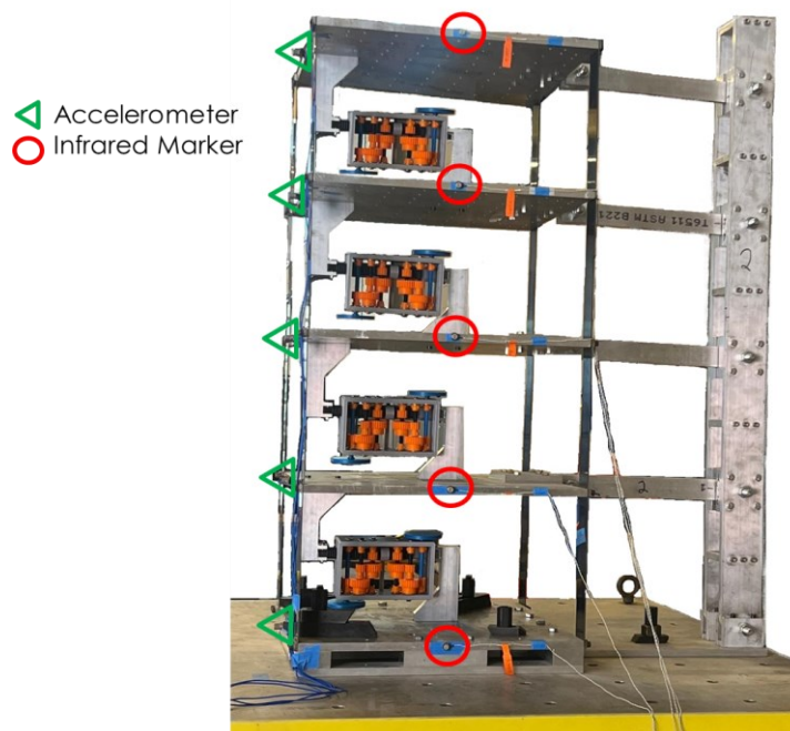
Figure 3. Physical model with instrumentation: accelerometers and infrared markers
