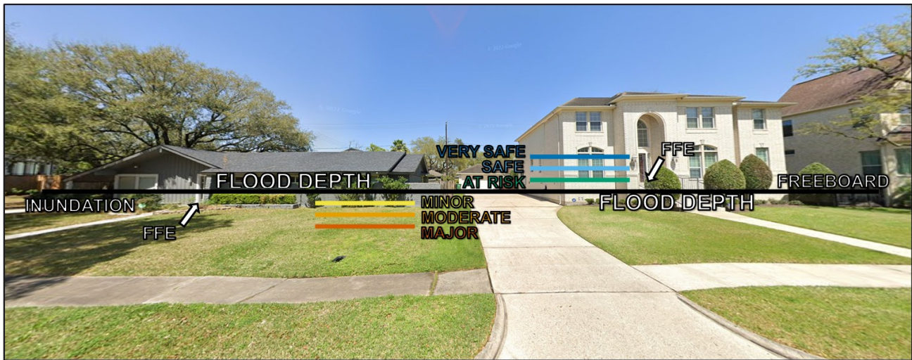
Figure 5: Example of vulnerability classifications on two buildings located in Meyerland. Image obtained through Google Street view. Schematic is for visual purposes only and is not to scale and is not for regulatory purposes.
