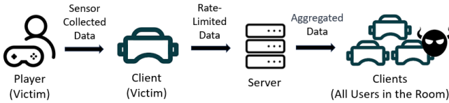
Figure 2: Motion data flow in multi-user VR applications.
