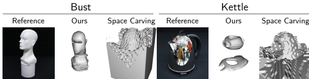
Figure 7. Because our reconstruction method assumes a Lambertian surface, it fails to reconstruct highly specular scenes, such as a glossy white bust (left) or mirror-finish kettle (right).
