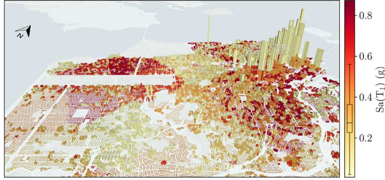
Fig. 3. Spectral acceleration Sa(T_1) of buildings in the San Francisco testbed, with building heights scaled in proportion to the number of stories.
