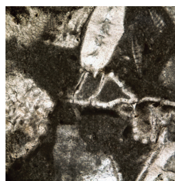
Figure F32. Nummulitic limestone with possible Morozovella spp. (398-U1589C-22R-1, 0–3 cm; PPL).
