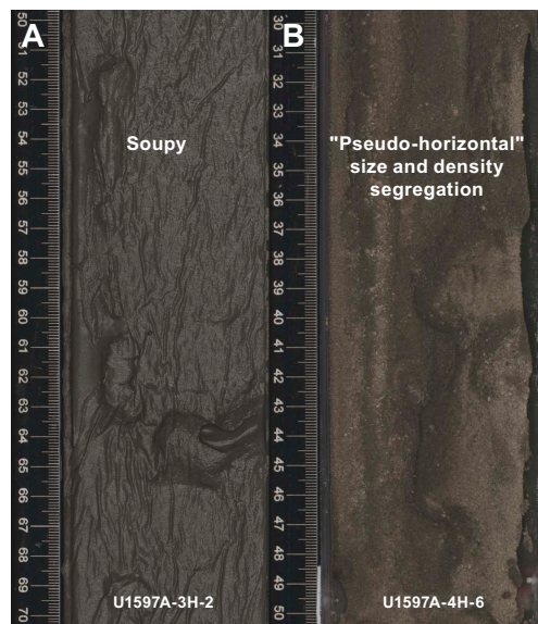
Figure F6. Core disturbances, Site U1597. A. Soupy ash. B. Artificial size and density grading or pseudohorizontal density grading caused by segregation of fine lapilli pumice clasts in liquefied sediments while the core is lying flat on the deck, resulting in vertical structures when the core is turned upright.
