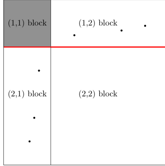
Fig.2. Illustration of the distance matrix in our proposed method. The (1,1) block is the anchor-anchor distance matrix. The (1,2) and (2,1) blocks are the anchor-mobile and mobile-anchor distance matrices respectively. The black dots indicate observed distance entries in these blocks. The (2,2) block is the mobile nodes - mobile nodes distance matrix. Grey indicates the distances are known in that block while white denotes the distance information is missing in that block. The red line indicates the last anchor node from which we know the distances to all mobile nodes.
