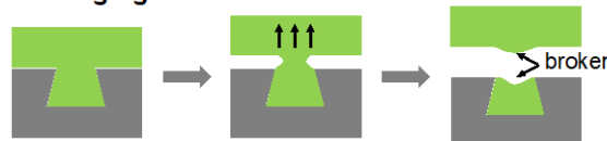
Figure 1: Comparison of demolding from different types of molds. (a) A soft structure (green) can be easily demolded from a mold with a pyramidal shape (gray). (b) A soft structure tends to be trapped in a mold with an overhanging shape. Successful demolding requires soft material with a larger size to be squeezed through a smaller opening.
