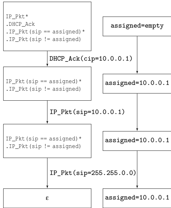
Figure 4: The progress of matching a string with the DHCP example. The left column contains the binding-free patterns, and the right tracks the environment. The arrows indicate the pattern derivative with the incoming event and current environment. Acceptance is indicated by the empty string, \epsilon .
