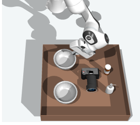
Figure 16: Illustration of a simple task and motion planning problem. The domain contains only one action: pick-and-place of objects. It contains three preconditions: g should be a valid grasp pose on object x , t should be a valid robot trajectory that moves x from its current pose to the target pose p , and during the movement, the robot and the object x should not collide with any other objects y . If successful, the object will be moved to the new location. The goal of the task is to pack both objects into the target box without any collisions.
