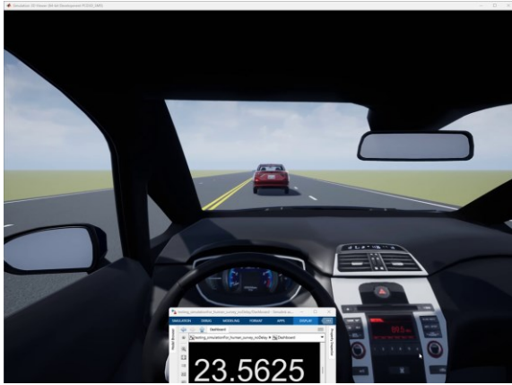
Fig. 14. Real-time display to the teleoperator during remote driving
