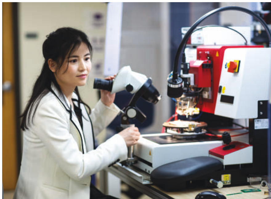
Professor Ruby Gu, director of the photonics program, demonstrates automatic wire bonder with pull/shear test capability.
