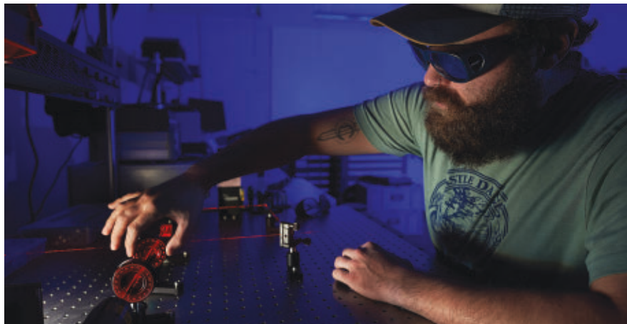
A student characterizing the properties of a polarizing beamsplitter.
