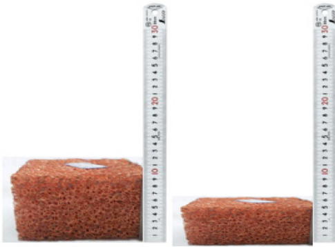
Fig. 2. Test metal foams of different thickness but same microstructure
