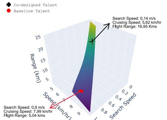
FIGURE 5: Talent Pareto front represented by Polynomial Regression applied to computed Pareto solutions obtained by multi-objective optimization of Talents; limits of talents captured with quantile regression.
