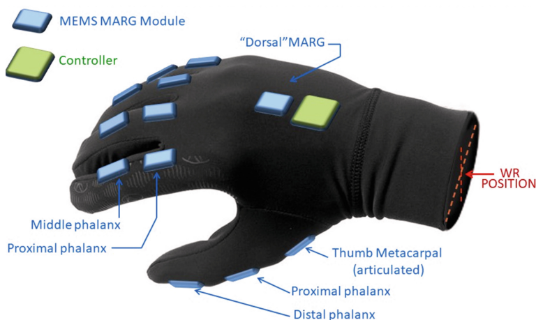
Fig. 1. Conceptual depiction of the glove, indicating the placement of the MARG modules. In the first proof-of-concept implementation two MARG modules are used to instrument the middle finger, two for the index finger and three for the thumb, in addition to the module placed on the dorsal surface of the glove.
