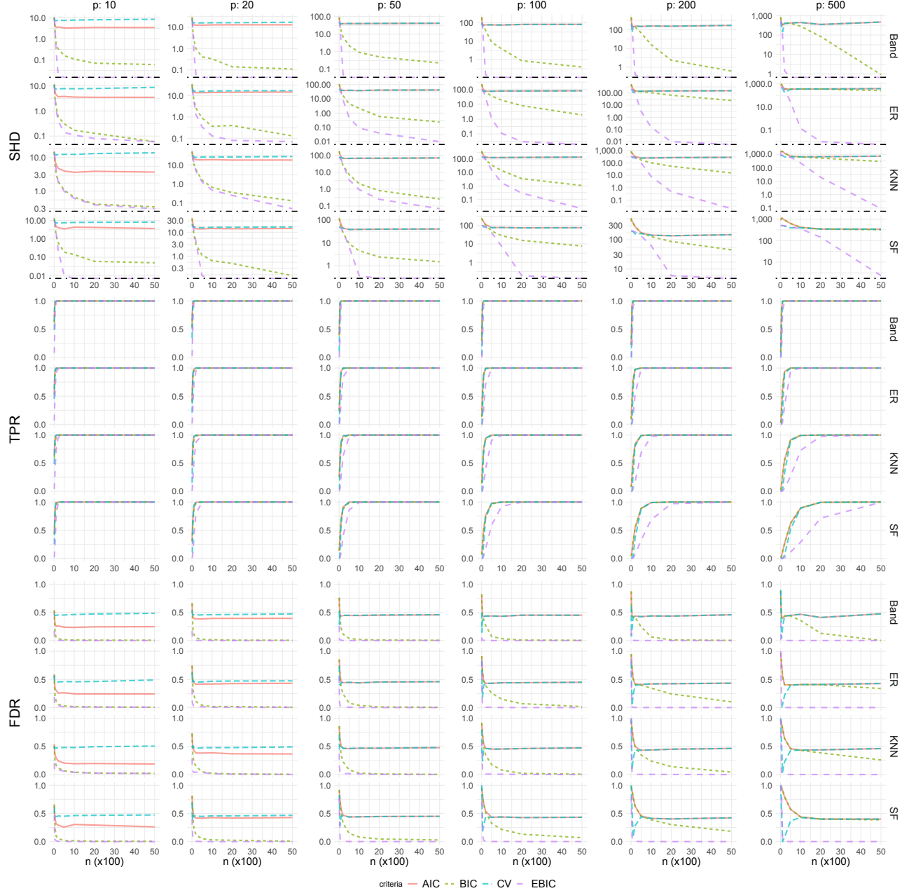
Figure 14: Average SHD, TPR and FDR over varying sample size n (in hundreds) and the number of variables p on groups of graph types using CLIME to compare criteria on 100 runs. The dotdash line represents the 0-SHD, i.e. perfect neighborhood selection. Wall time limit was set to three hours. Exceeding time limit or undefined FDR value for all zero estimates are marked as missing points for plotting.
