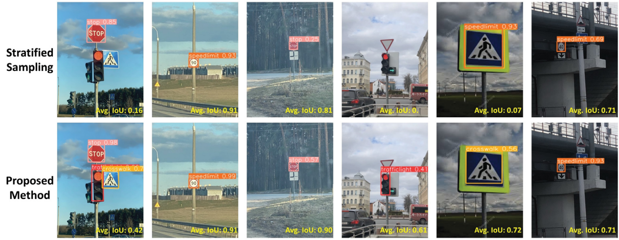
Figure 10. The application of our method in traffic sign interpretation. The selected results of detection by training a YOLOv8 detector from scratch using data selected by Top: Stratified Sampling and Bottom: Our proposed method. Our method demonstrates higher confidence and higher accuracy in the detection.
