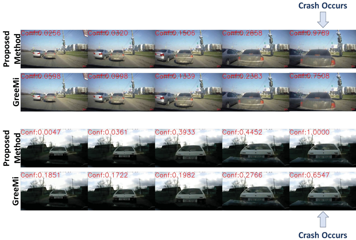
Figure 11. Video-based crash detection. Training videos are selected based on their frame diversity with respect to other videos using different methods. The confidence of the crash occurs provided by the attention map in sequential frames by two selection methods.
