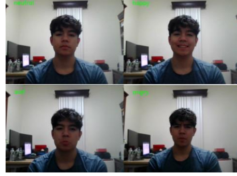
Figure 2: Example of emotion recognition by using DeepFace library.
