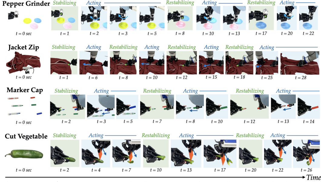
Figure 3: Experiment Rollouts: We visualize BUDS experiment rollouts. All tasks alternate between updating a stabilizing position w^s while the acting arm is paused and executing an acting policy while the stabilizing arm holds steady. We visualize both w^s and the acting actions.
