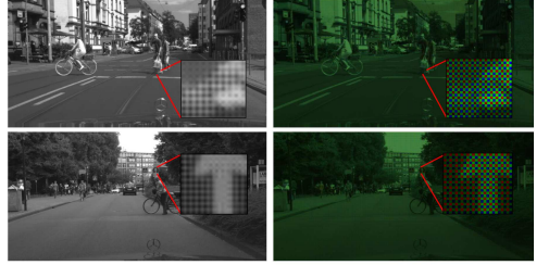
Figure 3: Formulation of raw Bayer images. For each sample image (row), left is the zoom-in 20 \times 20 pixels' region of the raw Bayer image; right is the raw Bayer image overlaid with color Bayer pattern for better observation.
