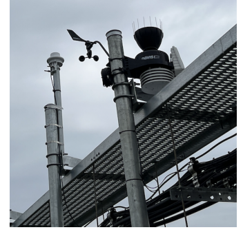
Fig. 3: Davis weather station (right) and OTT Parsivel Square disdrometer (left).
