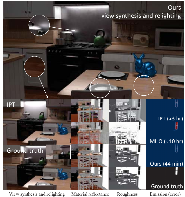
Figure 1: Ours vs standard IPT. IPT [1] takes a piecewise constant parameterization of material to reduce Monte Carlo variance and ambiguity for inverse rendering, losing fine spatial details as a result. Directly extending it to complex material representation (e.g. MILO [45]) shows very slow convergence. In contrast, we propose Factorized Inverse Path Tracing (FIPT) to get rid of variance and reduce ambiguities, yielding efficient and high quality BRDF and emission (4th row), appealing relighting (1st row), and object insertion (the bunny on the table). The presented scene is synthetic with the inset showing the input (lower-left sub-figure). We further showcase results on real scenes in Fig. 10 and 11.
