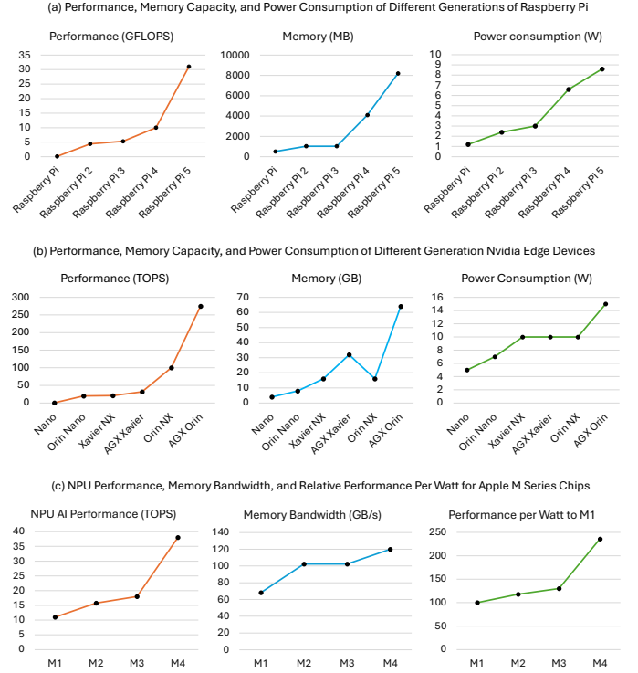
Fig. 2. Performance and Specifications of Representative Edge AI Hardware.
