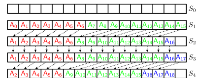
Figure 6: Priming an L2 cache set (writing A_0, \dots, A_6 followed by reading A_7, \dots, A_{15} ) and then accessing other addresses.
