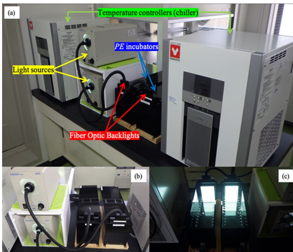
Fig. 3.2. An example of photosynthetron used for photosynthesis-irradiance (PE) incubations with two incubators connected to a light source and temperature controller; a) shows the complete setup, b) shows the front of the PE incubators, and c) shows the inside of the PE incubators.
