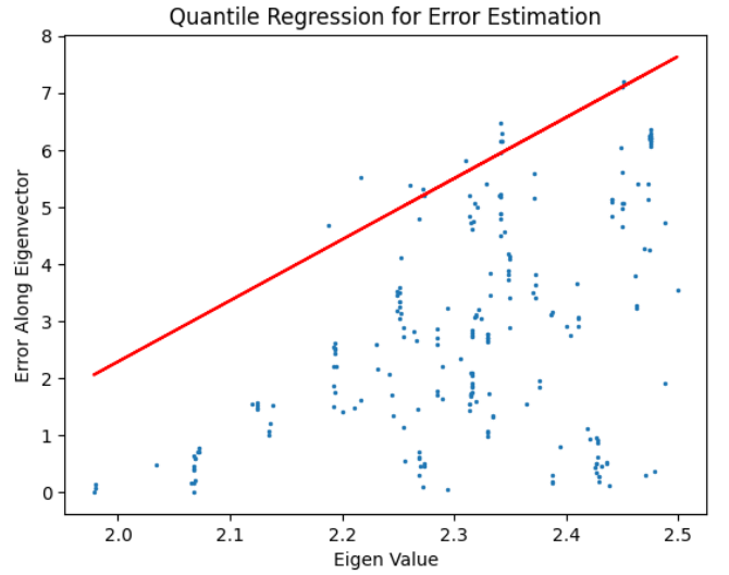
Fig. 6: 95% quantile regression line with eigenvalue-error pairs from SpotSpotter data. The eigenvalue-error pairs show an approximately linear trend in the 95% quantile as expected.
