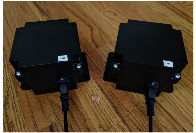
Fig. 2: Two low-cost (<$200 U.S.) gunshot detection devices each utilizing a Raspberry Pi 4 and a SPH0645LM4H-B microphone.
