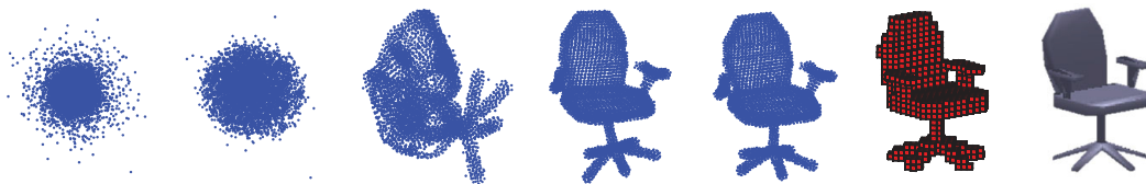
FIGURE 16. The self-organizing process of a recurrence network for the 3D design of a chair (YouTube video demo: https://youtu.be/FHI3eN5X6po ).
