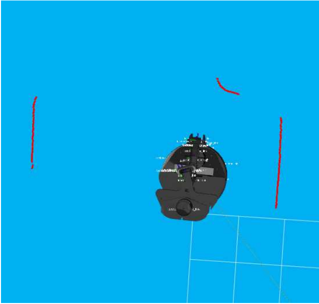
Fig. 5. The LoCoBot can detect its surroundings using a lidar sensor and process this data to show shapes and distances in RViz.
