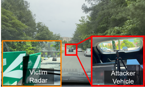
Fig. 17: Experimental setup for the moving vehicles studies.
