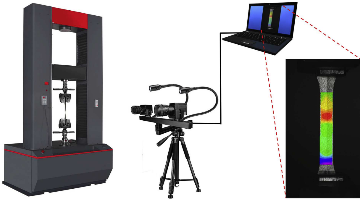
Fig. 1. Assessment of material deformation under tension utilizing a DIC. The setup features a testing machine that applies tensile force to the specimen, while the DIC camera system captures detailed deformation data. The resulting strain map highlights areas of strain concentration in various colors, processed by DIC analysis software.
