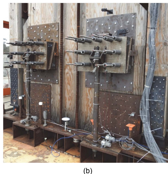
Fig. 4. (a) UFD schematic; and (b) installed UFD at West MPP wall.
