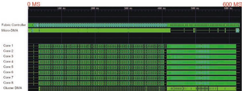
Figure 8. A trace of the network that accepts 250x225 images shows that the GAP8 processor's cluster cores are underutilized. The green line segments represent periods of activity, whereas the gray line segments and unshaded portions represent periods of inactivity.
