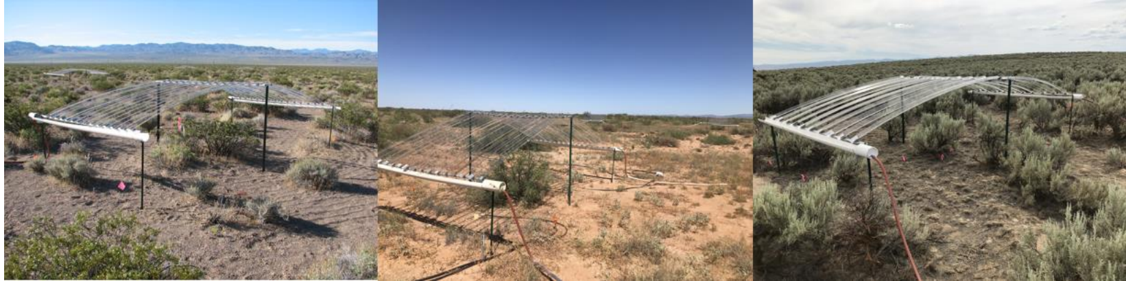
Figure S3.1.1. Photographs of rainfall exclusion shelters at the Mojave, Chihuahuan, and Great Basin sites in this experiment (left, center, and right respectively). Plots were centered over individuals of the dominant shrub species at each site.
