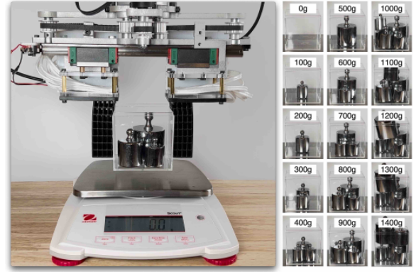
Fig. 7: Experimental setup for sensing different weights. (Left) For each of 7 pre-defined grasp strengths, the gripper makes 3 attempts to grasp a box filled with weights. digital scale confirms a successful lift-off. (Right) The experiment is repeated with 15 weights from 0 to 1400 g.
