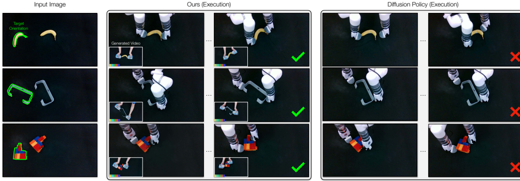
Figure 4: Rotation Qualitative Results. For this task, we provide as input the image on the left for each row, with an example of a successful rotation overlaid. Our video generation-based approach succeeds, while Diffusion Policy fails to select stable grasping points on the object, causing it to slip during manipulation. Generated videos are indicated by ■ ■ ■ .
