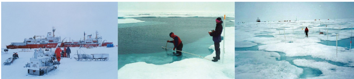
Fig. 13 The SHEBA expedition had an extensive multidisciplinary sea-ice program. Left: autonomous platforms were deployed to monitor the meteorological, sea-ice, and oceanic conditions. Middle: Routine measurements of lateral ice melt were conducted for investigations of sea-ice mass balance. Right: Networks of ice thickness gauges enabled continuous monitoring of sea-ice mass balance. Photographs courtesy of Don Perovich.
