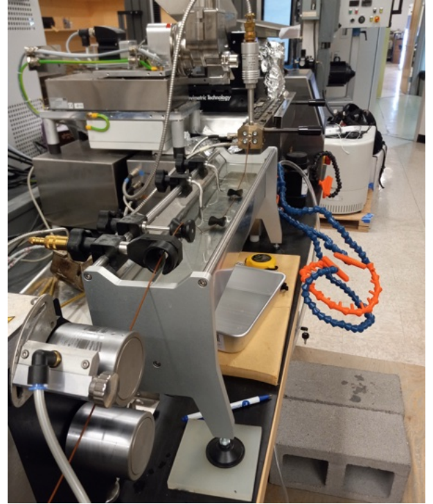
Fig. 1. Manufacturing process for the filaments via Twin-Screw Extrusion
