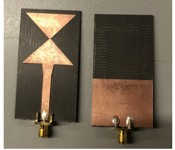
Fig. 2. Milled bowtie antenna, From [14].
