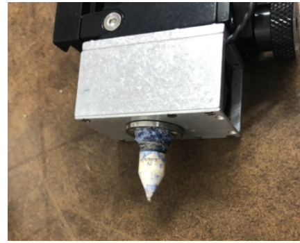
Fig. 7. Filament overflow due to nozzle clog.
