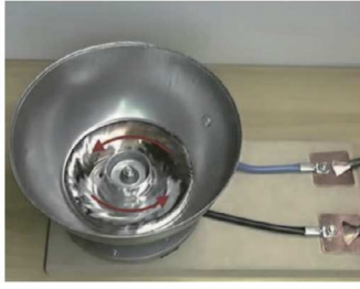
(a) Comparison of an experimental photograph of a liquid mercury rotator with the calculated velocity field \mathbf{u} and magnetic field \mathbf{m} at t = 1.2 .
