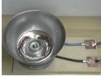
(b) Comparison of an experimental photograph of a liquid mercury rotator with the calculated velocity field \mathbf{u} and magnetic field \mathbf{m} at t = 1.2 , after reversing the applied magnetic field.
