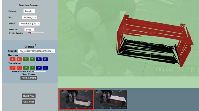
Figure A10: The interface for manually adjusting part poses in 3D. The interface supports adjusting the 3D position and orientation of each part. The interface also provides visualization of the 3D parts from different perspectives.
