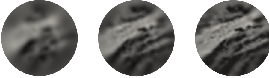
FIG. 9. (Ice sheet) The log basal friction parameter, with color scale as in Figure 8(b), computed from the PDE-constrained optimization problem with noise levels: 25% (left), 5.0% (middle), and 1.0% (right).
